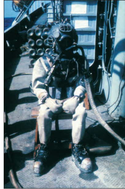
Figure 1-15. MK V MOD 1 Helmet.
